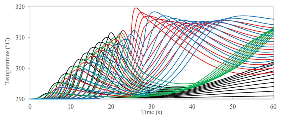
MS temperatures for the four panels (black 1<sup>st</sup>, red 2<sup>nd</sup>, blue 3<sup>rd</sup> and green 4<sup>th</sup>) during the filling procedure (until the 25<sup>th</sup> second) and switch to normal circulation (each panel is divided into many longitudinal cells)
