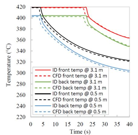
Metal internal and external temperatures in the back and front sides of the tube during the filling procedure at different axis coordinates
