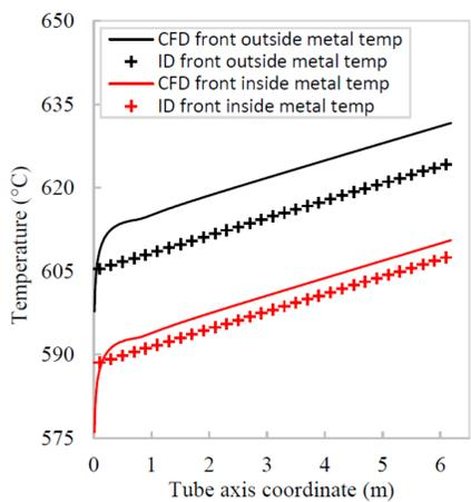
Metal internal and external temperatures in the front side of the tube with a constant flow rate of MS (steady state) as a function of the axis coordinate
