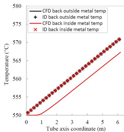
Metal internal and external temperatures in the back side of the tube with a constant flow rate of MS (steady state) as a function of the axis coordinate
