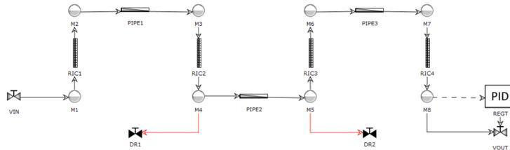
A basic model of a receiver system has been built in ISAAC Dynamics in order to test in a more complex system the behavior of the pipe previously analyzed. A simple regulation system consisting in a single PID varies the valve VOUT lift in order to change the MS flow rate and obtain a MS outlet temperature of 550 °C
