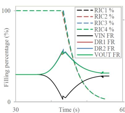
Panel filling percentages and draining valve flow rates during the drainage procedure of the receiver.
