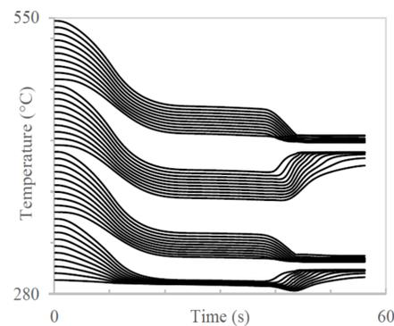
MS temperatures for the four panels (each panel is divided into many longitudinal cells) during the drainage of the receiver
