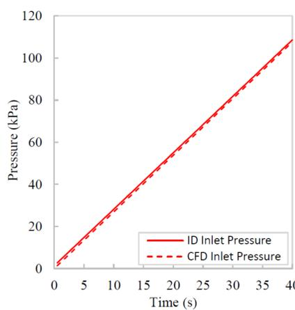
Pressure at the tube inlet necessary to guarantee a constant flow rate during the filling procedure as a function of the simulation time
