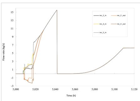
Full trend of each panel mass flow rate. After the complete filling of the receiver system (with the receiver outlet valve in closed position), the PID takes control of the flow rate in order to keep the MS outlet temperature at 550 °C
