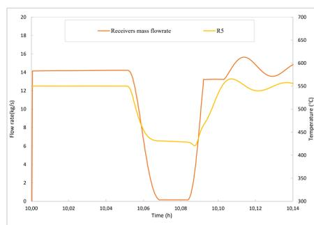
Total shadowing of solar field. The absence of solar irradiation is extended for 120 seconds; the regulation system tries to keep the outlet MS temperature at 550 °C by lowering the MS flow rate. In total absence of DNI the MS flow rate is lowered to a value close to zero in order to avoid the MS temperature degradation inside the receiver. When a regular DNI is restored, the regulation system increases the MS flow rate to nominal values
