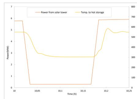
(1) A cloud generator was applied for about 1 hour; the regulation system tries to keep the receiver outlet MS temperature at 550 °C varying the rotational speed of the feed pump and the lift of the hot storage tank inlet valve. (2 and 3) When highly opaque clouds last for a long time, the by-pass valve opens and, simultaneously, the main hot storage valve closes. After the passage of the cloud, the system switches to nominal state condition restoring the base receiver control system
