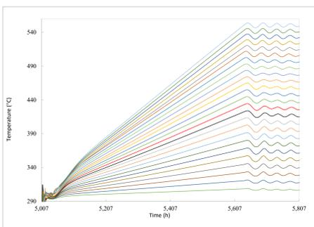
MS Temperature in the receiver for each panel. In the first phase of normal circulation, the control system waits for the MS to reach a certain temperature before controlling the outlet valve. In the right side of the figure, it can be observed how the flow rate regulation system impacts all the MS temperatures in the panels
