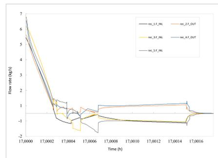
MS flow rates during the drainage of the receiver; panels number 1, 3 and 5 show negative flow rates when the cold pump is no longer able to support the MS weight and, in that moment, they start to drain
