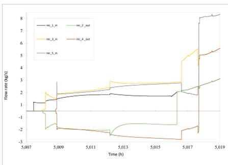
The figure on the side represents the MS flow rates in the five panels during the filling of the receiver; the difference among the flow rates in each panel is due to the geometrical asymmetry of the receiver. Negative flow rates in panels 2 and 4 are due to the MS flow direction opposite to the normal circulation
