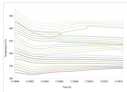
Temperature of the MS in each panel during the drainage procedure. The thermal behavior of panels 3 and 5 is quite interesting to analyze; in fact, they share the bottom manifold with panels 2 and 4 respectively; these two panels contain colder MS with higher density and, for this reason, they will drain easier. MS is kept for a longer time in panels 3 and 5 where it loses more energy to the environment.
