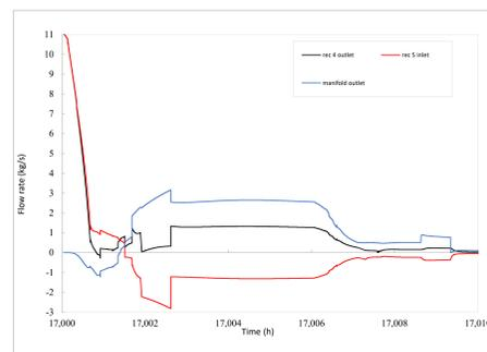
It's interesting to analyze the trends of the flow rates in the bottom manifold shared between the panels 4 and 5. When the flow rates of the panels decrease, they create an aspiration of the MS present in the outlet line of the manifold (blue trend). Only when the panels flow rates are close to zero the drainage can begin.
